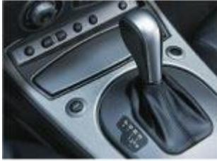
A gear shift lever enables the driver to select the desired driving mode. This lever can be operated using at least four different positions, identified by the letters P,R,N,D (**P**ark, **R**everse, **N**eutral, **D**rive). In case of shift levers equipped with a manual mode M (**M**anual), the driver is given the ability to shift manually by pressing the "+" button for upshifts and the "-" button for downshifts.
